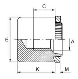
Female thread A = M6Height K = 11.0Min thread length C = 6.0Outer diameter E = 13.0Plate thickness = 4.1 to 4.3
